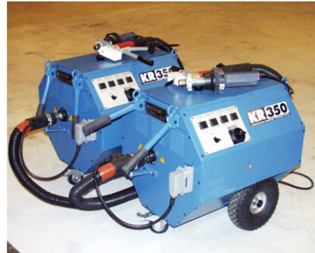
Figure 30: Krah Welding Extruder with flexible hose output 10kg/ hr.
