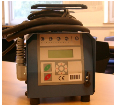
Figure 31: Tiny Data: Krah electro-fusion equipment, for E-Fusion sockets from 300 mm up to 4000 mm
