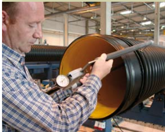
Checking of the wall thickness
