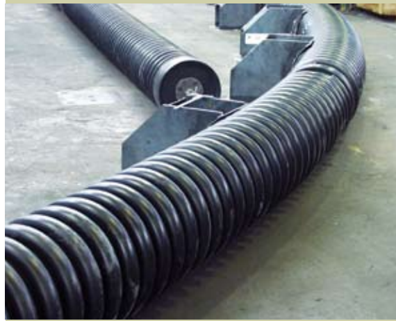
Bending of Krah pipes R/D = 30
