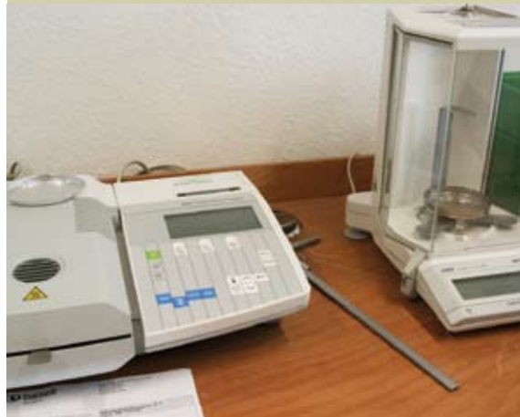
MFR-testing and moisture testing
