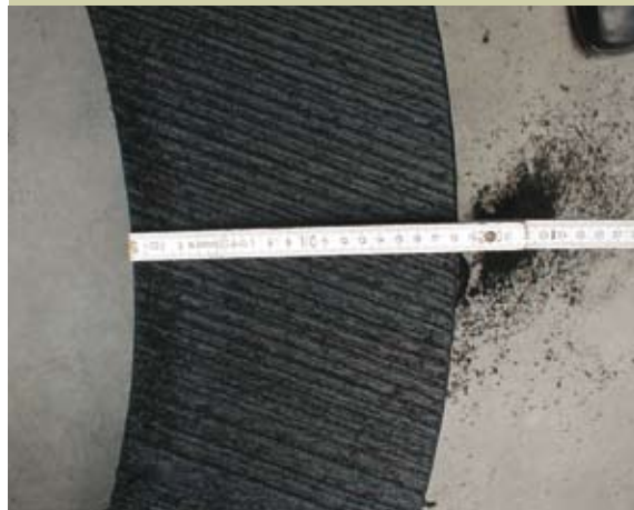
Solid wall polyethylen pipe, s = 180 mm
